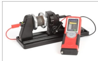
IP/Resistivity Module with Small Sample Holder
