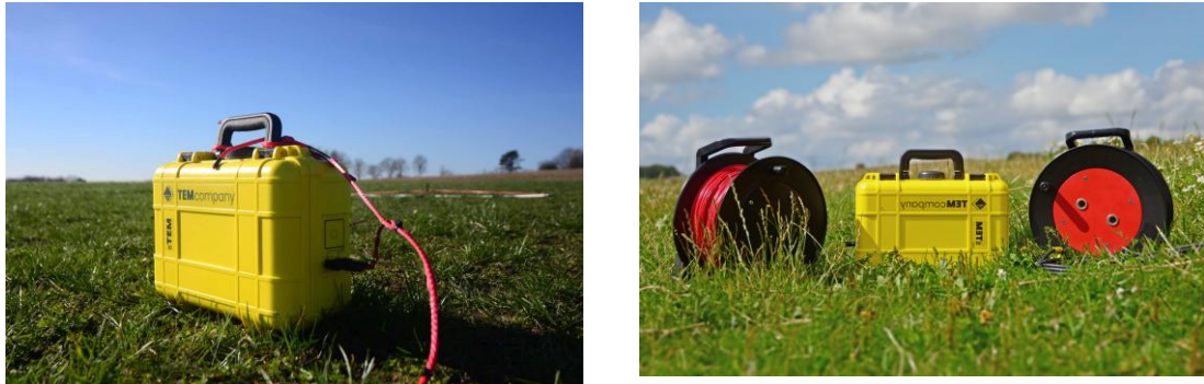
Figure 3 the picture shows the sTEM unit and the transmitter and receiver drums.
